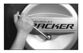
Using the wheel wrench, remove the wheel cover nut. Gently pry the spare tire cover off the wheel.
